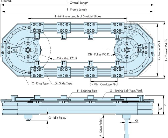
A system with 180° ring segments in an oval circuit is shown above. Rectangular systems with 90° segments are also available.
